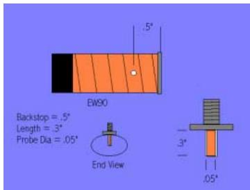
ter of .05" and a conductor length of .3") into a hole drilled .5" from each end of my 95' ength of waveguide. I then soldered a brass plate on each the end of the waveguide. Proper deaning and the use of rosin solder flux will assure proper solder flow with minimum heat!
