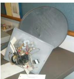
higher bands, with several prodly showing off their 24GHz setups, each unique in their parts and structure. At left is the handiwork of AA3GN, using a small offset feed dish and feed arm as a platform, a weatherproof endosure for the electronics, and a big waveguide switch as the
